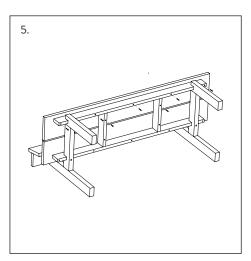
5. Spread out a rug/towel on the ground to protect the bench. Then, carefully place the Peka Bench on its back. Attach all seven of the small wooden screws into the corresponding holes on the underside of the seat.
