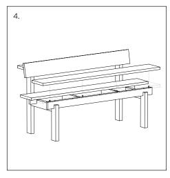
4. Attach seat - Part B using two of the long wooden screws. Make sure to match up the protruding dowels with the indentations in seat - Part B.
