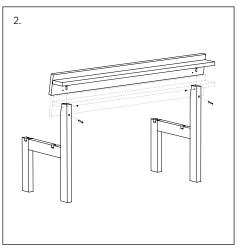
2. Place the two legs upright. Attach the backrest using both of set screws and both of the machine screws.
