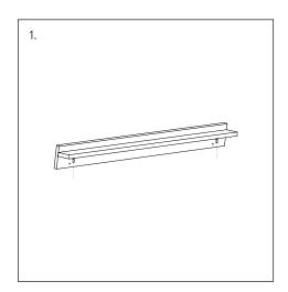
1. Mount the two bolts onto the underside of the backrest's shelf.
